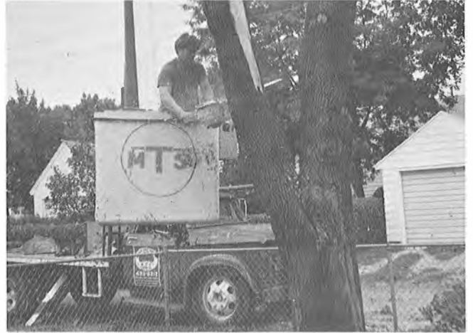
Now the same job is done with chain saws. The man in the bucket can raise, lower or move his position so that he is in the exact position for easy cutting.
