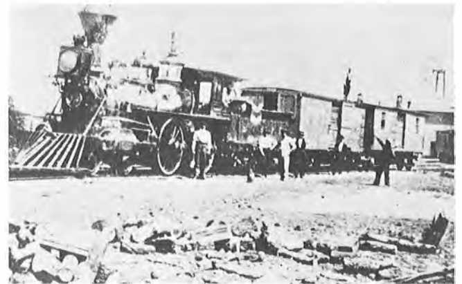
Two views of first train in Austin. The wide smokestack was used for wood burning locomotives. (Davison Photo)
