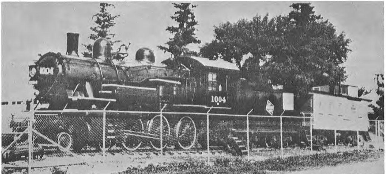
The 1004 began life as a class B-4 4-6-0 (Baldwin, 1901). It was rebuilt at the Milwaukee Shops in 1920 and emerged as No. 2604, a class G-8 and received the current number in 1938. The 1004 holds the distinction of being the last active steam locomotive on the Milwaukee. It was steamed up to handle the Austin-La Crosse passenger train (Nos. 158 and 157) on March 16, 1957. A month later it was retired from active service and soon thereafter placed on display at the Mower County Fairgrounds in Austin. (Davidson Photo)
