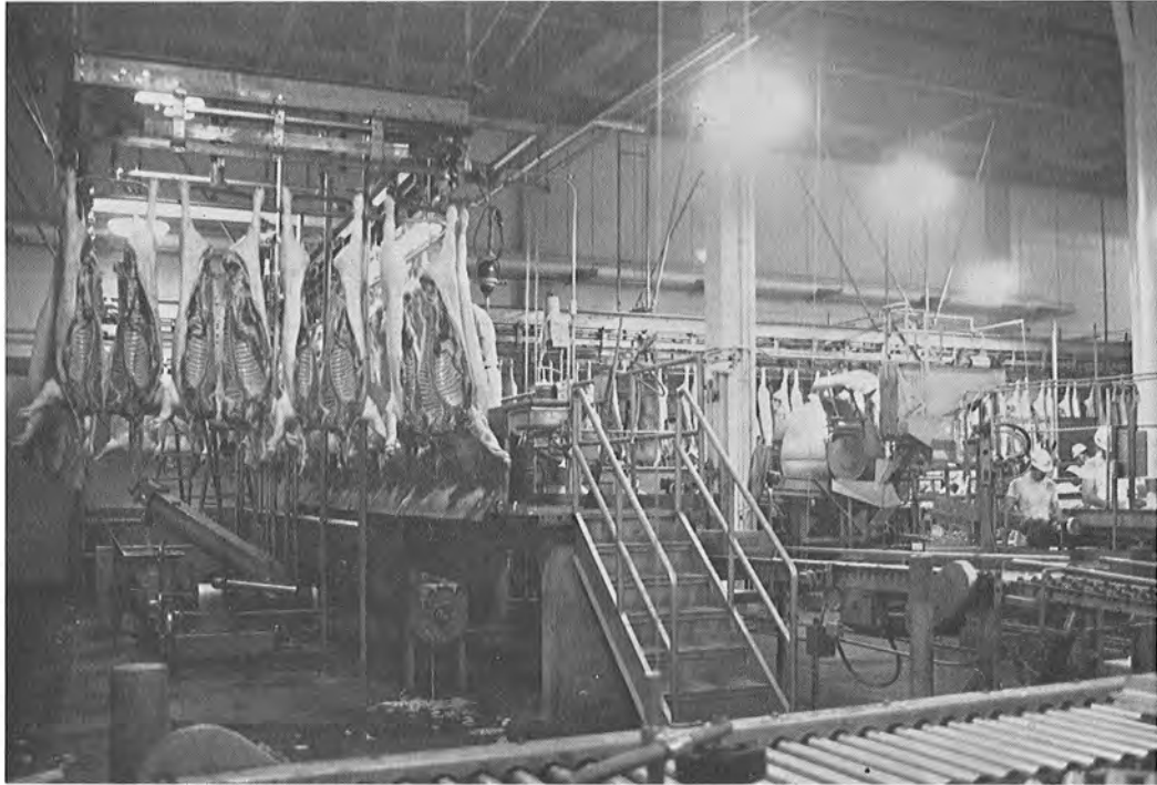
About 750 hogs per hour, or in excess of two million hogs annually, will be slaughtered and processed in this modern abattoir area. Facilities for hog slaughtering and processing are located on all four levels of the plant.
